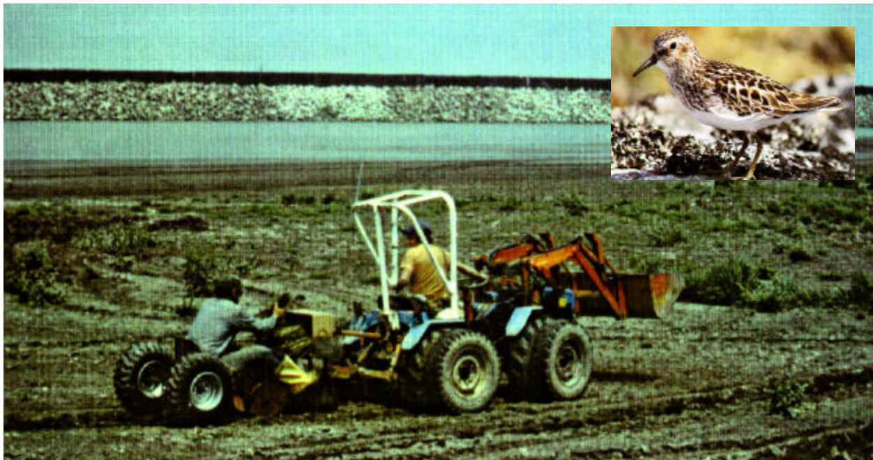
A three-point-hitch modified strawberry planter was used with a Pasquali tractor to plant cuttings and rhizomes in the relatively consolidated portions of the dredged material. Inset: a least sandpiper.
